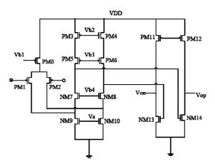
Fig. 1. The main operational structure
